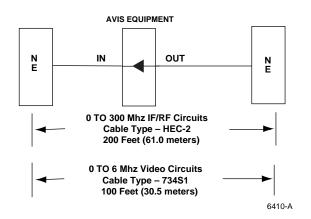
Figure 11. Recommended Maximum Cable Lengths
